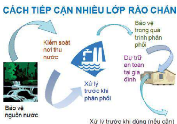
Figure 1: Innovative Multi-layered Barrier Approach to safe water management
