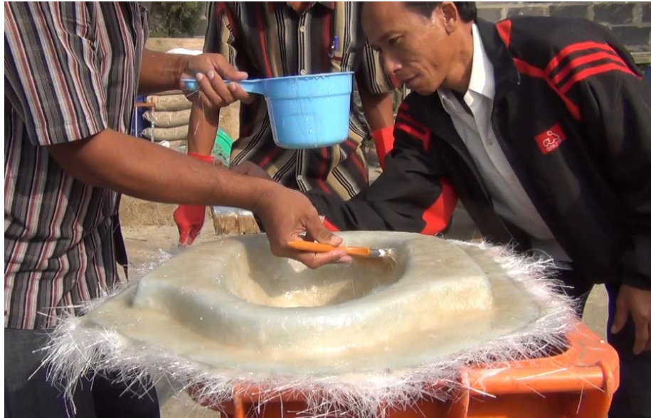
Making mold from composite material
